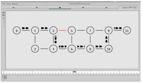
Figure 3: Fast Reroute one-to-one backup model.
